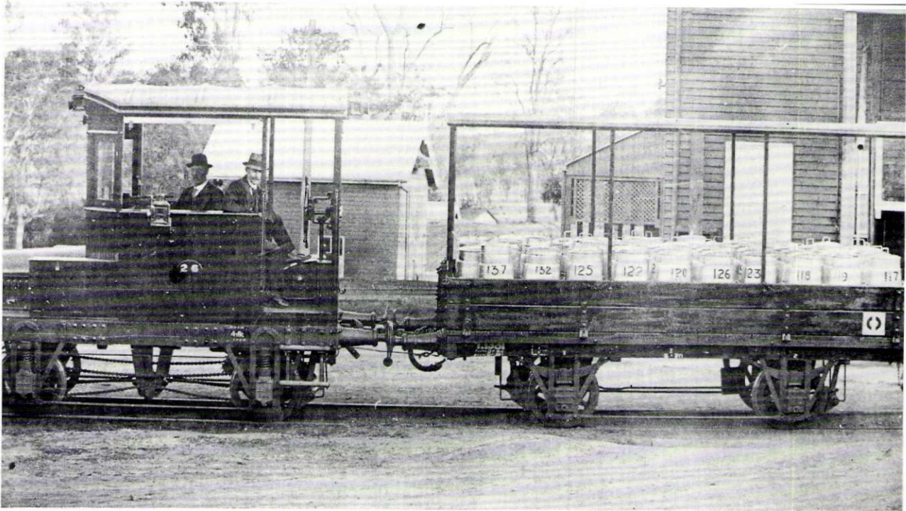
Napier 35HP Railmotor which transported milk from Linville to Nestle's Toogoolawah condensery in 1921-1922. John Oxley Library
