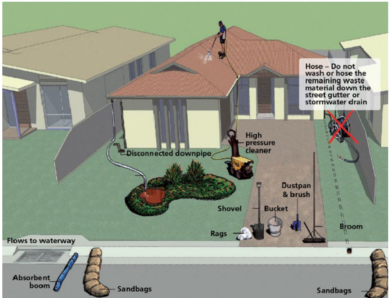
Artist impression of an acceptable setup for roof cleaning and restoration with downpipes disconnected and wastewater directed to a garden.
